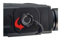
Fig. 6 open battery cover
