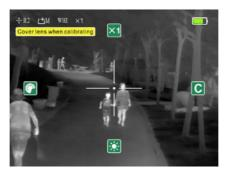
Fig. 21 the background calibration interface
