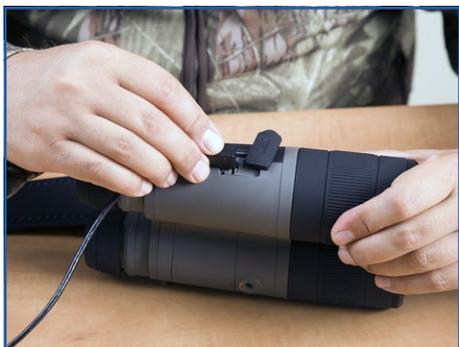
Insert the microUSB plug in to the microUSB media port.
