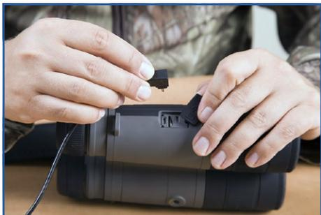
Depending on the device you have, you would either lift the rubber media port to expose the media slots. Or unscrew the media port cap if using with the ATN OTS-X HD.
