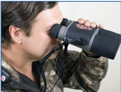
You are now ready to turn "ON" your ATN Smart HD device using the external battery pack as a power source. Press the "POWER" button on your device to boot the system.
