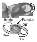
To maximize battery life, set the LCD Display to the minimum brightness setting practical.
