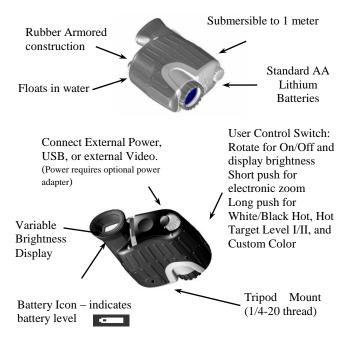
Serial Number is behind the external connections plug
